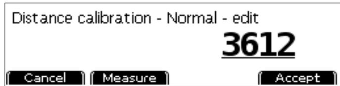
*Calibration screen for normal (pulse/reverse) sensor in Eltrip-65nce*
