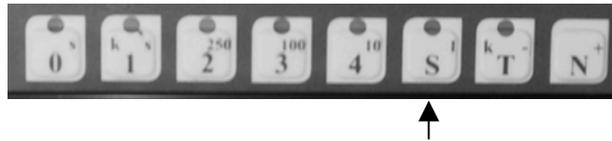
If you want to turn the display off, keep S-button down for approx. 2 sekonds. The display and all the leds turn off simultaneously. The counters operate normally.
