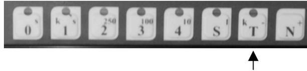
Step 1. Push down the T-button once if you want to select the reading of the time counter onto the display. The "time" LED on the right hand side of the display will illuminate. Time is in the form of hours and minutes.
