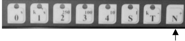
**- - - If your ELTRIP includes the friction measurement (ELTRIP-45nk), you are now in the mode for setting the coefficient value. In other case this will move you to the normal measuring mode.**
