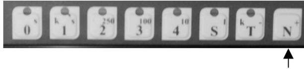
Step 1 Push down the button of the counter (0...4). The reading of the counter 0 ... 4 is on the display
